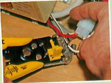
You'll need a qualified electrician to make the 12V power connections. This clever Würth cable stripper removes insulation from the length of the earth cable ready for a soldered connection.
