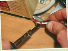
The negative connection to the 12V socket was made by soldering the stripped end of a sufficiently heavy cable as a kind of T-piece. The joint was then insulation-wrapped.
