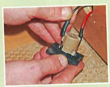
Here's the shape of the back of the socket. The connectors have been protected from electrical contact with shrink-fit insulation. The tube is slipped on, heated – and it shrink-fits!
