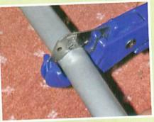
Cut right through in one smooth movement. It pays to look after the blade because it's easily damaged if used for levering or for cutting inappropriate materials.
