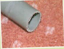
This is a piece of 20mm pipe used in houses for water storage tank overflows. Here is what happens when you cut using a hacksaw - a frayed finish.
