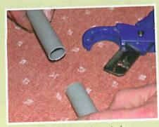
You can see that the cut pipe, whether drain or water pipe, is smooth and ready. On some cutters a blunt blade can be reversed and new ones are easily fitted.
