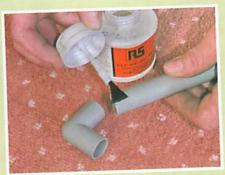
Rigid PVC pipes are best welded together, though this does mean you can't get the joints apart later. The weld will permanently damage many other plastics if it touches them.
