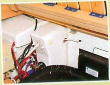
Use the correct size of hole saw or a (tapering) stepped drill but don't make the hole too big. Here, the aerial cable attached to the socket is passed through the hole...
