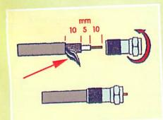
Prepare the cable as shown, twirling the braided section (arrowed) and wrapping it back, around the insulation. Push and screw on the Fplug connector, making sure the centre protrudes as shown.
