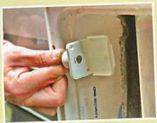
If possible, fit the socket inside the battery box. There's a waterproof cap, but even so... The aerial wire can pass through the recess for the mains cable.
