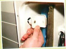
...and the aerial socket, with the flap open, is pushed into position. If you're fitting it outside the battery box, the socket flap hinge should be at the top.
