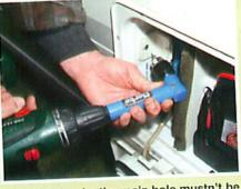
Here's why the main hole mustn't be too big. You need to drill pilot holes near to the edges of the main hole. This inexpensive Clarke angle adapter is a real boon!
