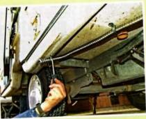
The exhaust pipe must angle backwards from the direction of travel and exhaust at the edge of the caravan, keeping gases away from any openings leading to the interior.
