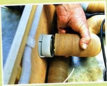
The Truma-type vents we used were fixed in place. Each one consists of two parts and afterwards the hose was simply pushed in. It self-grips on the grooves inside the vent.
