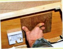
Our caravan's bulkhead consists of insulation sandwiched by thin sheets - too thin for screws but the charger must be screwed down. Plywood reinforcing was then taped and screwed into place.
