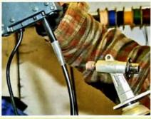
In our case, the 12V cable on the charger wasn't long enough so we extended it, using soldered connections (another electrician's job!) and protected the joint with Würth heatshrink tubing.
