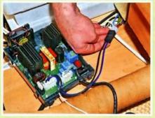
If the caravan's existing 12V plug is the standard type, all you have to do is plug it in to Socket 1. If not, have an electrician fit a new one.
