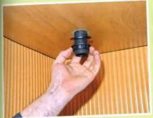
Inside, the mast tube is held with a rubber washer and screw-on flange. The hole for this tube absolutely must be drilled upright - check with a spirit level when drilling.
